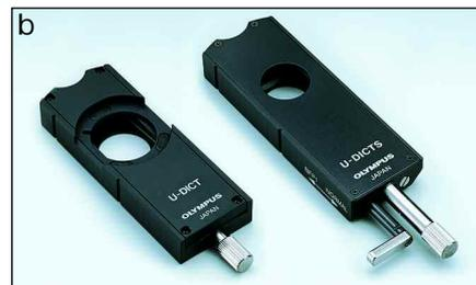
(b) DIC sliders which are inserted into the nosepiece of Olympus BX microscopes. The lefthand slider has a recess to accept an analyzer.
